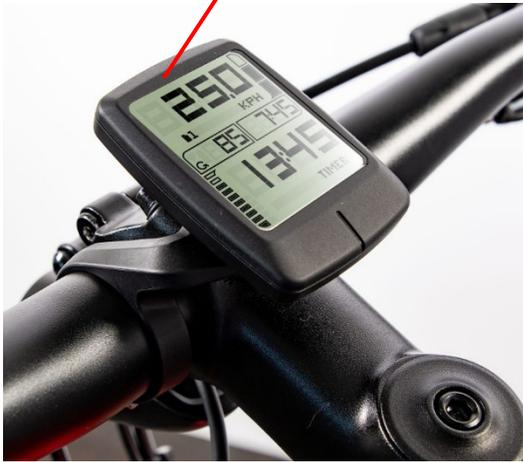
All Turbo Vado/Como Bikes with a TCD-w have the ANT+ module built into the display.
