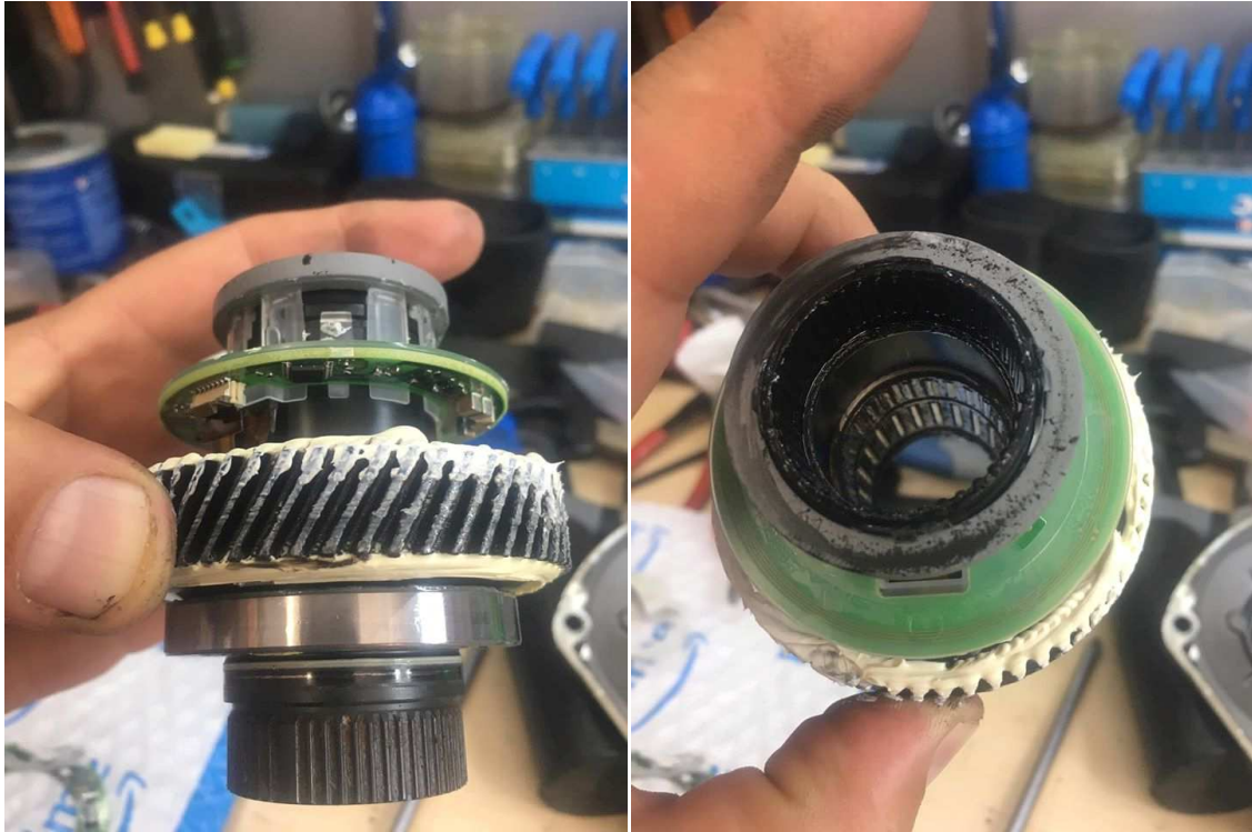
The main shaft with the roller bearings, where the bottom bracket is inserted
