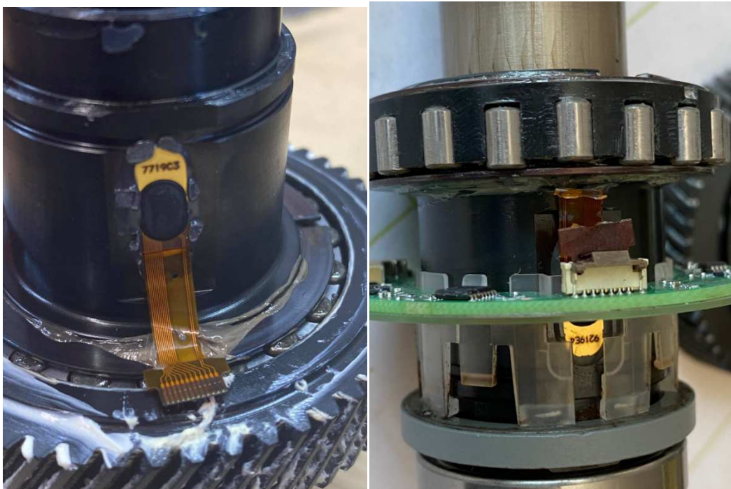
In the first photo we see the torque sensors that are of the "Strain Gauge" type and are bonded to the shaft with putty. In the second photo we see the rollers of the Sprag- clutch which us inside the black sprocket.
