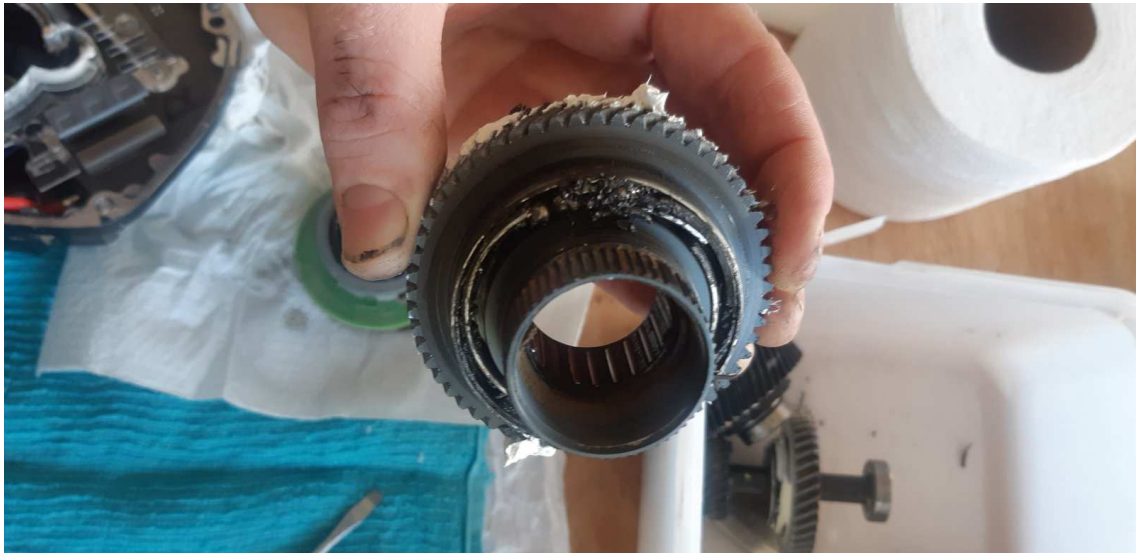
Damaged Bearing and below the damaged bearing housing in the motor case
