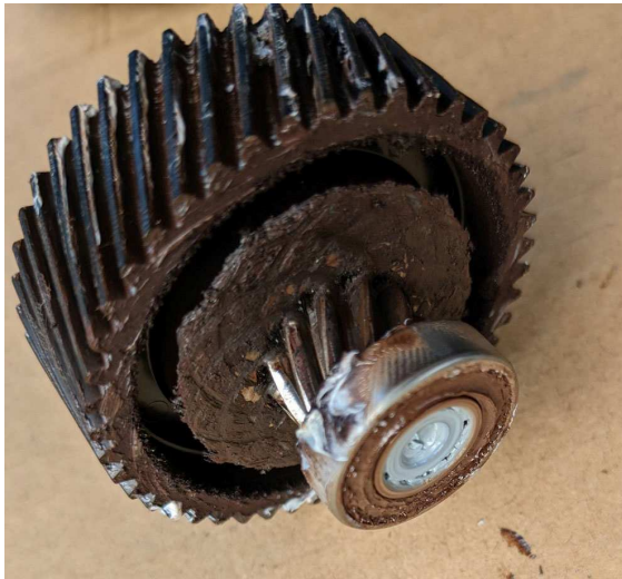
Sprocket with degraded grease transformed in gum:
