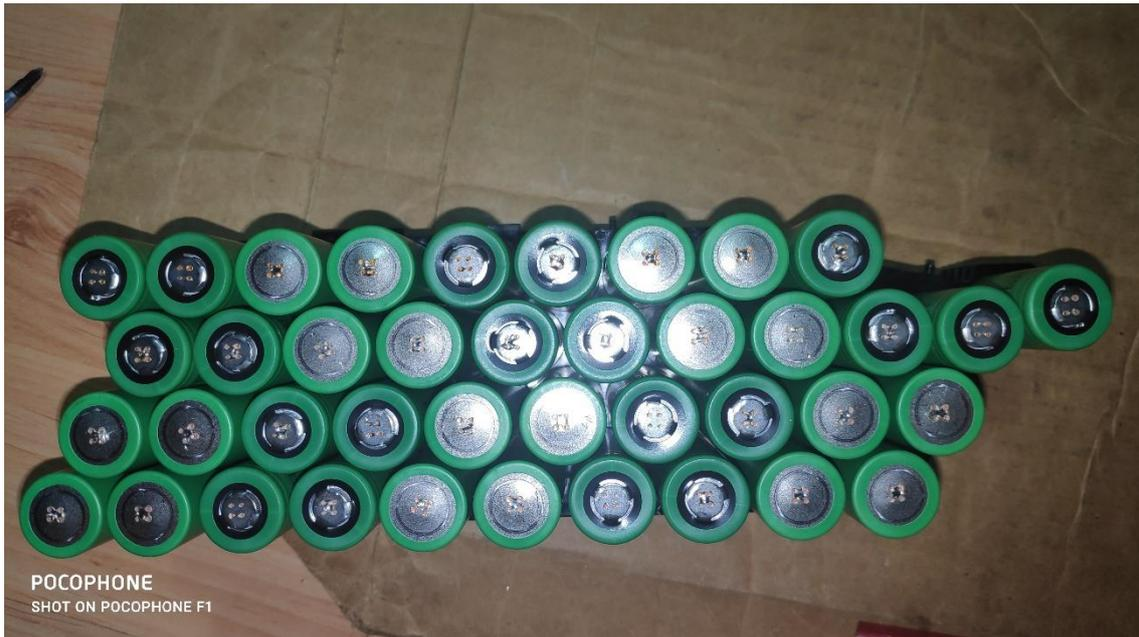
We will place our new cells, I chose the 3500mah Samsung 35E cells. They can be placed from other brands, as long as they meet the condition of being 18650 format, and that they have a capacity of 3400-3500 mah
