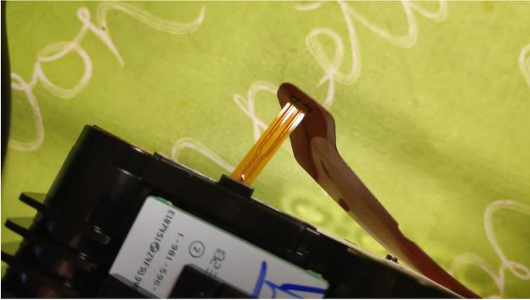
Now if we have completely isolated the electronic board of the BMS with the cell block.
