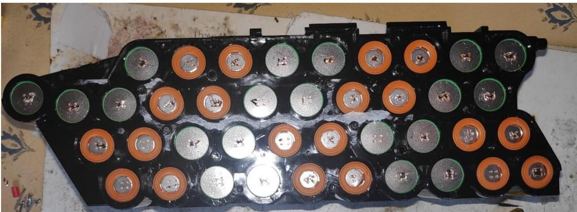
Once all the dangerous nickel strips have been removed. We proceed to remove all the screws that surround the entire contour of the plastic casing, where the cells are housed.
