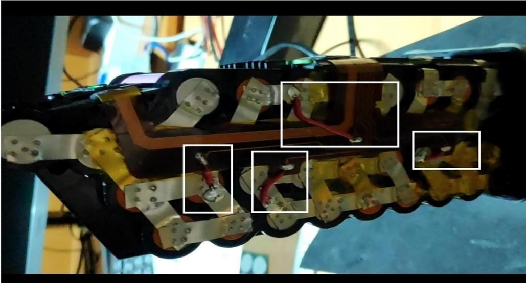
In conclusion, adjust the plex strips, under the channels through which the outer shell must slide. We don't want to rip them off when we try to slide the casing off.
