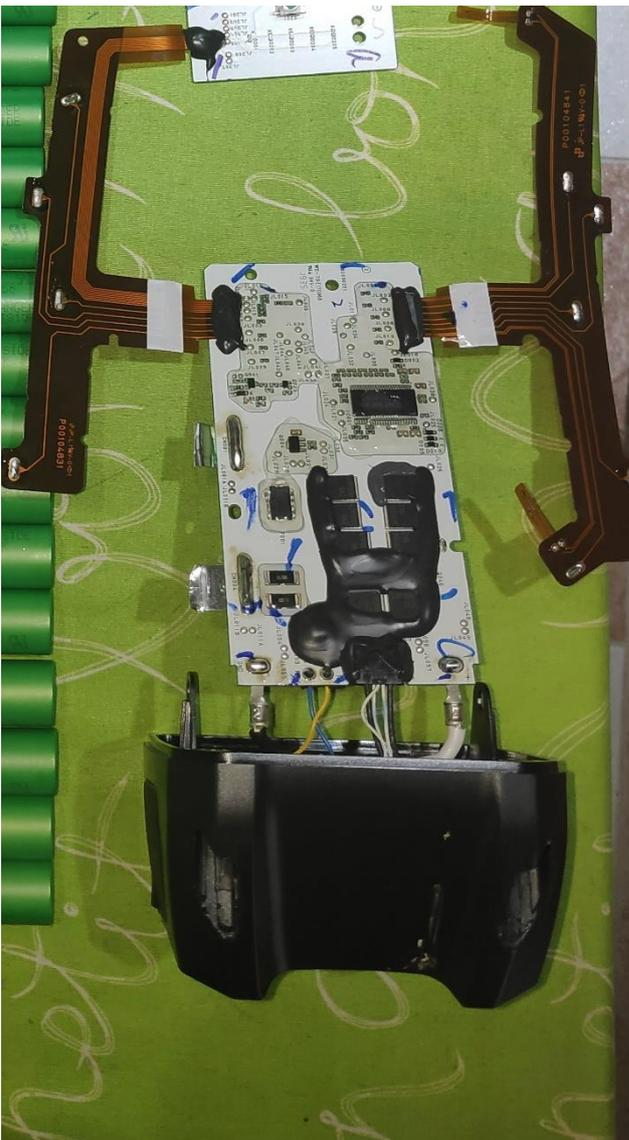
It is advisable that on the back of the flex, we place some small stickers on the welding points. To perform the insulating function. It will make our work easier when we reconnect the flex with the new block of already restored cells.
