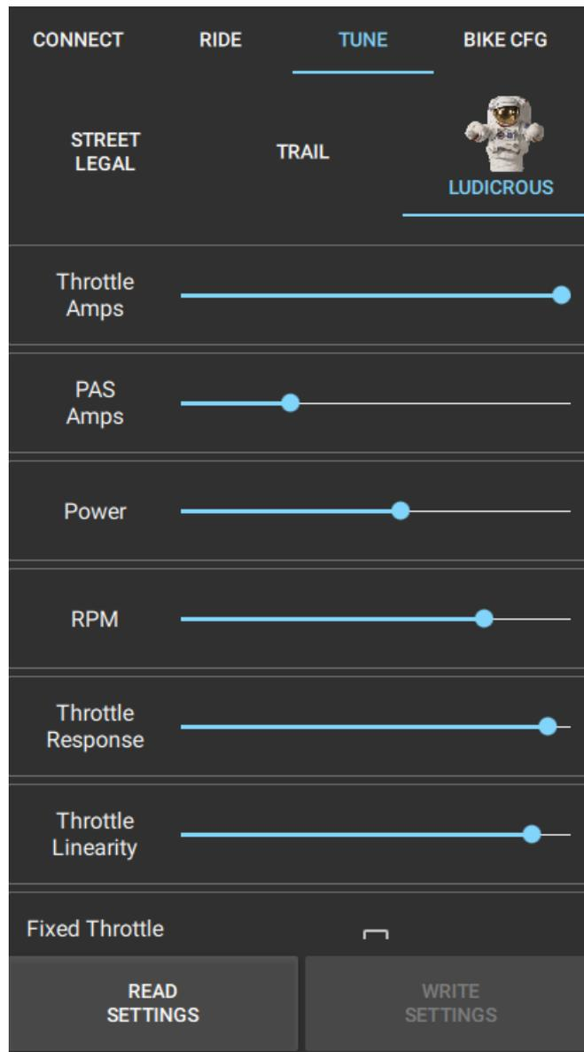
By tapping the **WRITE** button, the selected profile will be stored in the controller.
