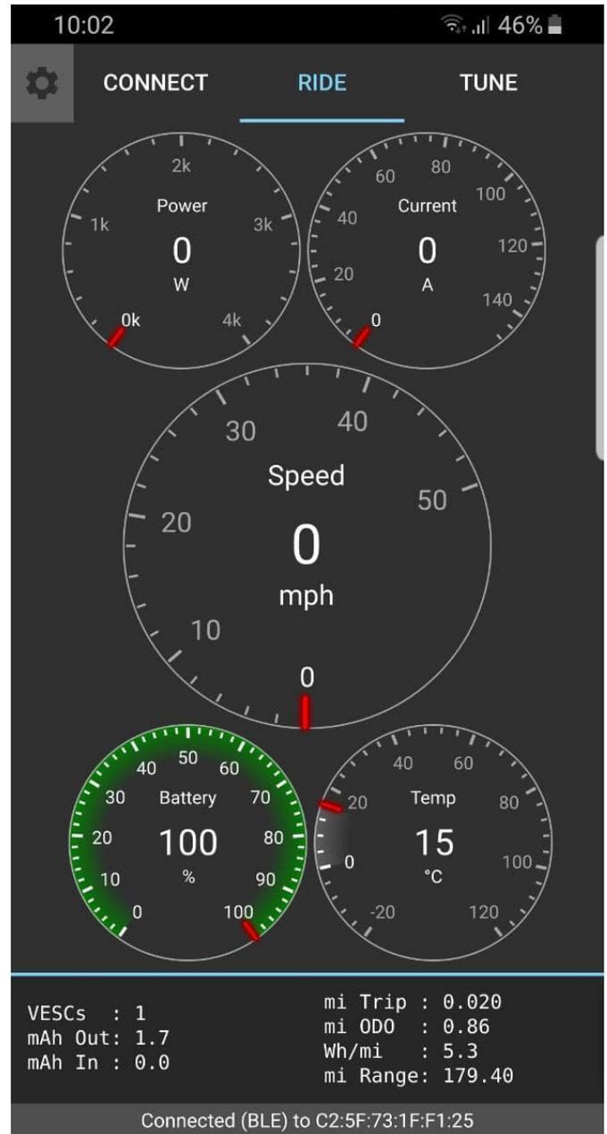
4. In the RIDE tab you can see live data coming from the controller. We added a Motor Temperature gauge, as the Ludi V2 can easily drive the motor to its temperature limits.
