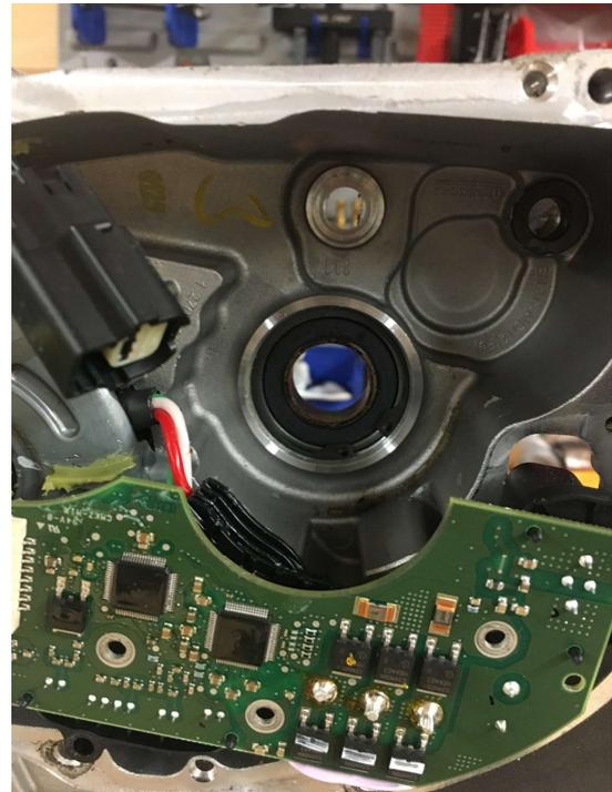
One of the first things I noticed was the main motor drive gear needle roller bearing had worn the needle rollers to the point that the roller cage that supports the needle rollers was starting to wear
