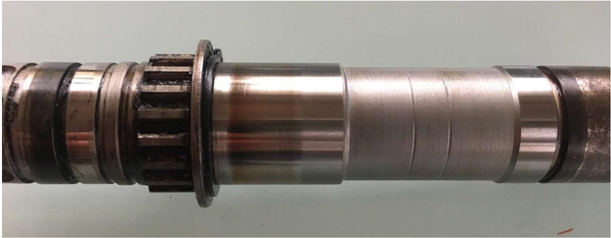
There were very little signs of wear to most of the metal and plastic gears, although back-lash (play) could be felt by rocking the crank back and forth. Some of this may have been caused by worn clutch bearings. Although, is more likely the wear of the gears overall.
