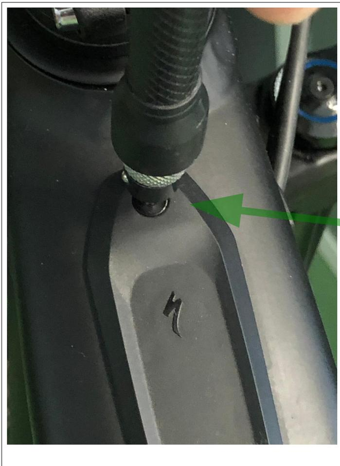
**Unscrew the screw holding the TCU to the bicycle.**
