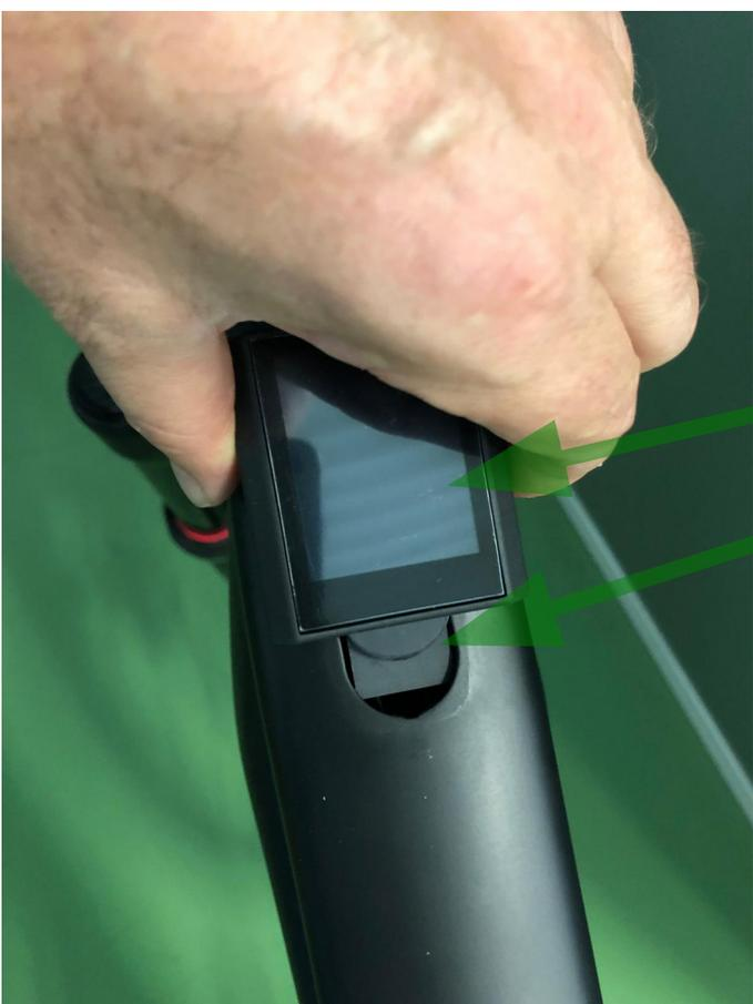
After having made all the cables enter the tube, insert ADAMO19 inclined, making sure that the rectangular tongue will enter the tube, while the round one must remain external. Upon insertion, it will be slightly forced, but still use the utmost delicacy. Help yourself with a thin metal strip.
