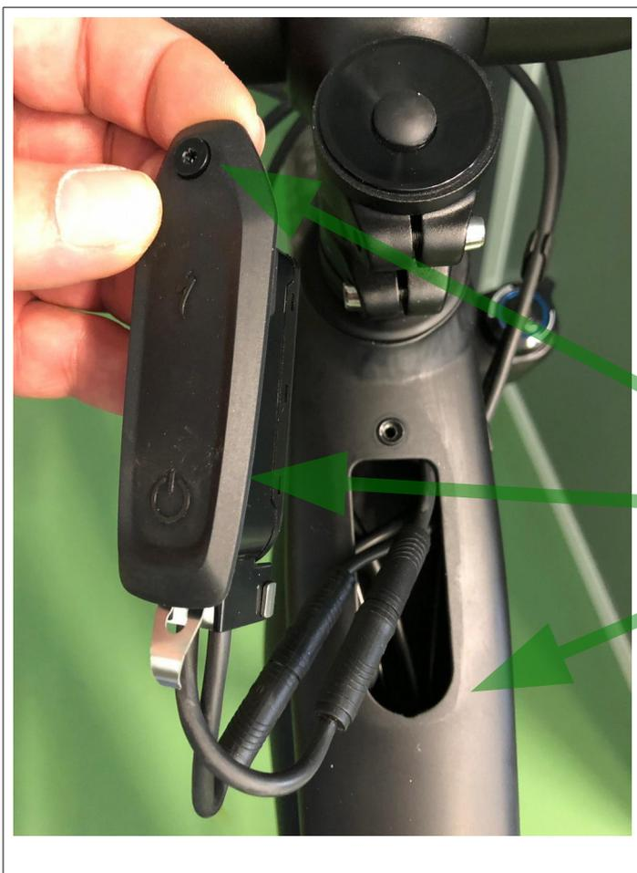
**Remove the TCU from its housing and be careful not to lose the screw.**
