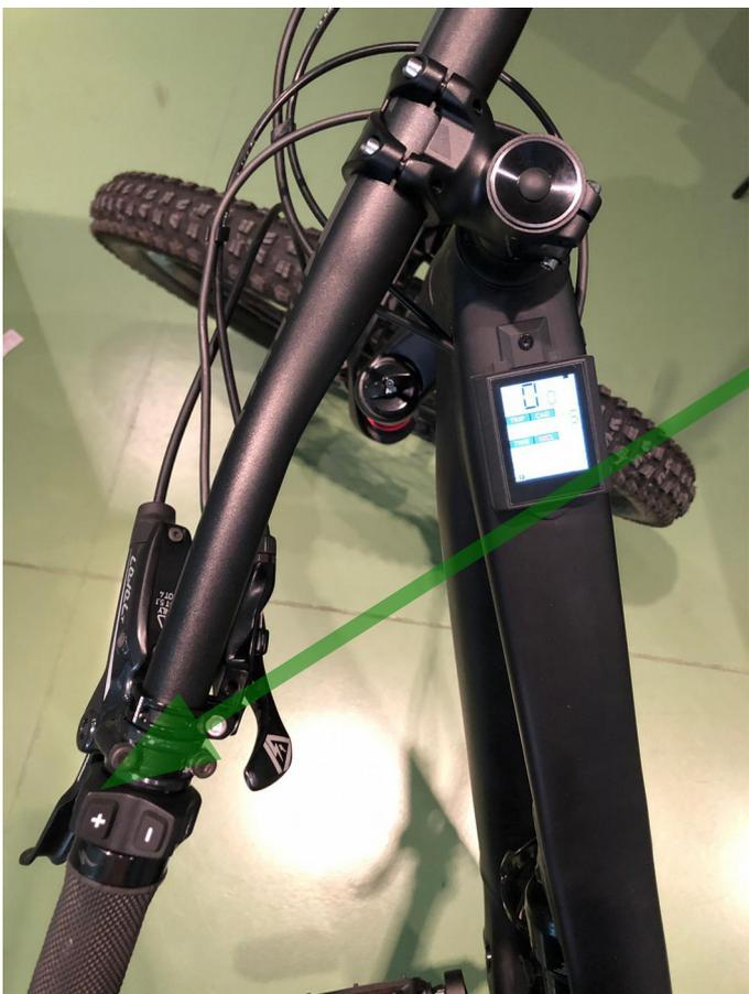
**When everything is finished, keep the TURBO button pressed for a long time to turn on the bike and check that the display is on.**
